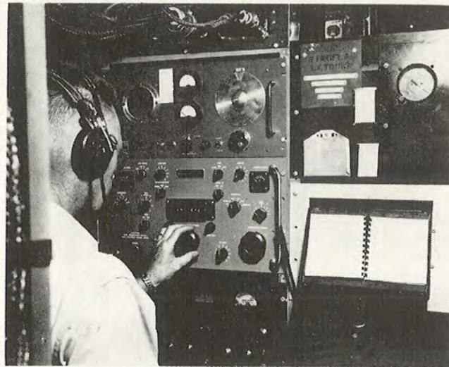
Frequency monitoring equipment in the B-25 aircraft.
